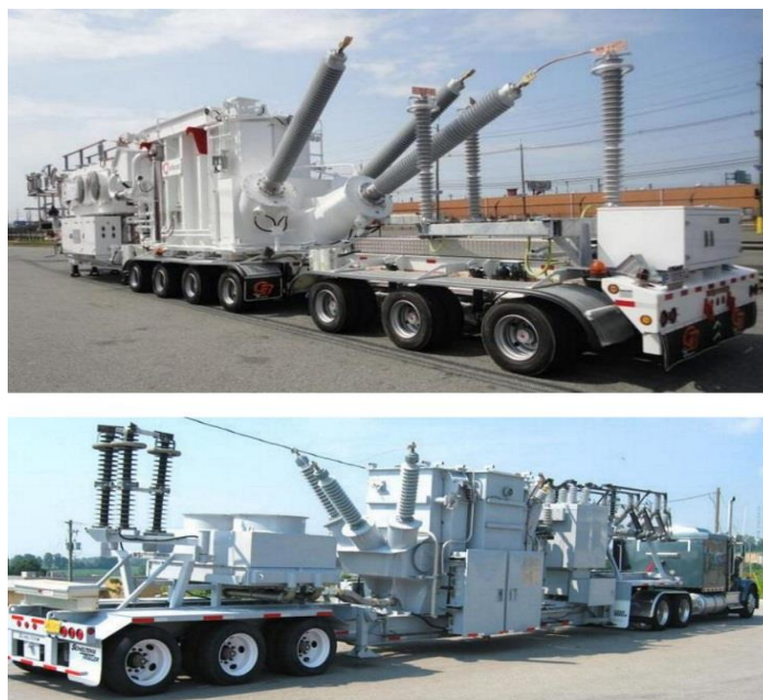
Fig. 1. Several types of mobile substations
